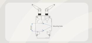
**3. Mounting the Base Station:** Place the base station on a flat, horizontal surface, or mount it against a vertical surface using the mounting holes underneath the device. The mounting slot accommodates 3 mm screws.
