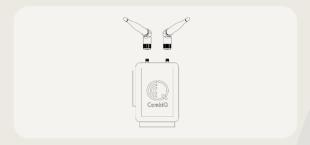
**1. Attach LTE Antennas:** Attach the LTE antennas to the SMA connectors on the back of the base station. The maximum tightening torque is 0.9 Nm.
