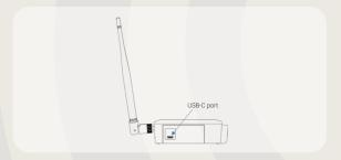
**4. Connect the Power Adapter:** Connect the supplied power adapter to the USB-C port on the side of the base station, and then plug the adapter into a 230V wall socket.
