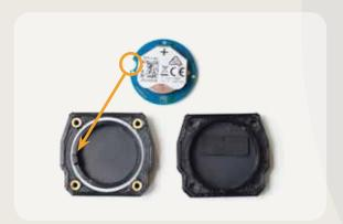
**2. Cover Assembly:** Fit the circuit board with the lower part of the cover, aligning it with the arrow in the image. Tighten the screws to ensure the cover is secure.
